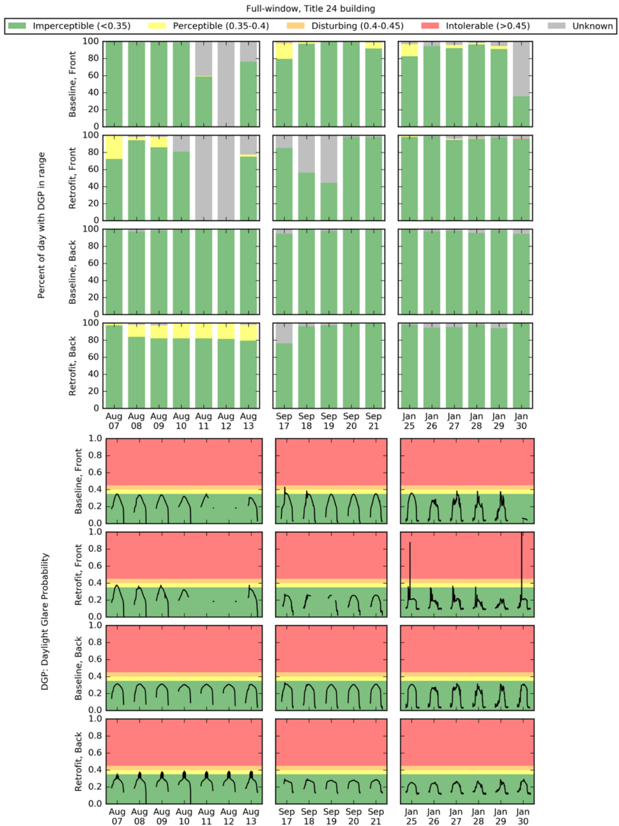
Figure 33. Full window code-compliant building baseline Daylight Glare Probability results
