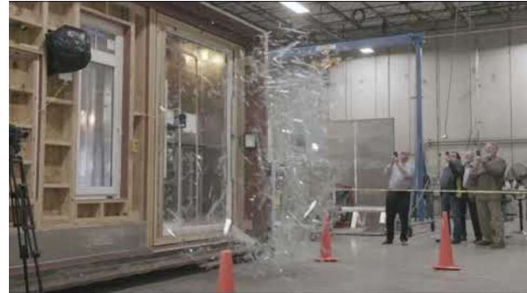
Outer pane shattered before thinglass at 240mph windspeed (50 ft 2 glass unit)
