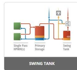
Primary plant with a temperature maintenance plant in series
