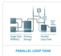
Primary plant with a temperature maintenance plant in parallel
